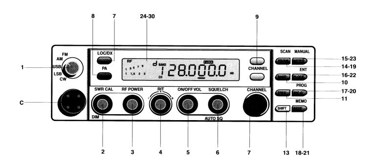
**1. Mode switch.** This control is used to select the desired transmit mode. The modes available are: CW, LSB, USB, AM and FM.
