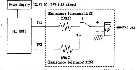
Set the switch of the Anneter jig at 1 position, adjust L502 to 25 µ Å reading on the DC Anneter.
