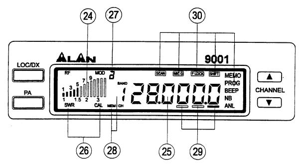
24. **MULTIFUNCTION METER-** This meter can display S/RF, Modulation, SWR Cal, or SWR. See the section on operation for more information on using the multifunction Meter.
