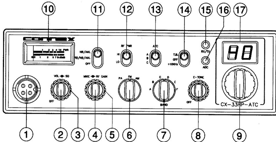
1. **MICROPHONE JACK:** Used to connect microphone for voice source.
