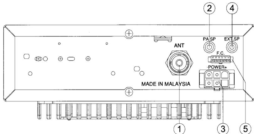
1. **ANTENNA** : This jack accepts 50 ohms coaxial cable with a PL-259 type plug.
