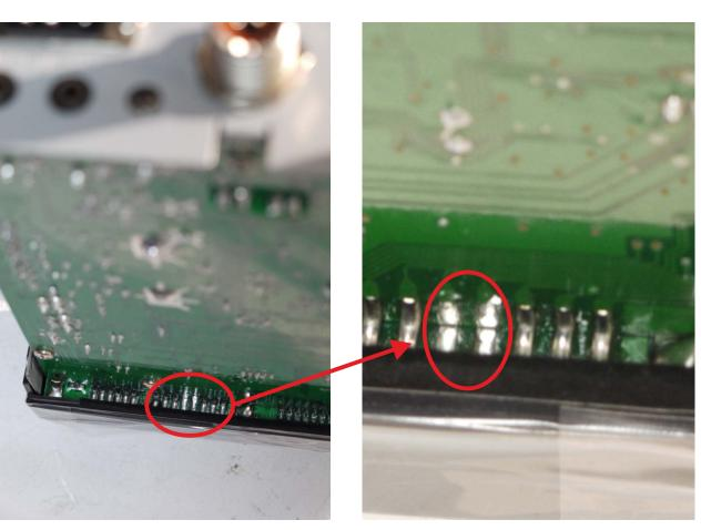
These two points must be soldered for transform into CB 400 Ch
