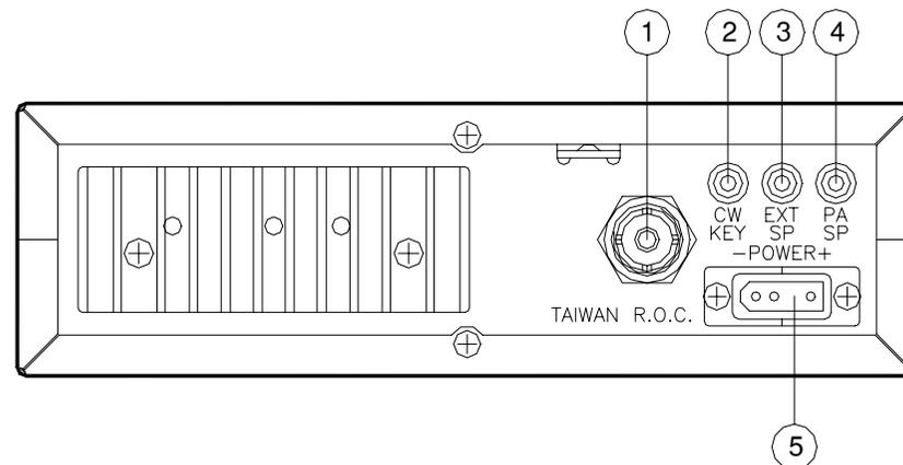
1. **ANTENNA:** This jack accepts a 50 ohms coaxial cable with a PL-259 style plug.
