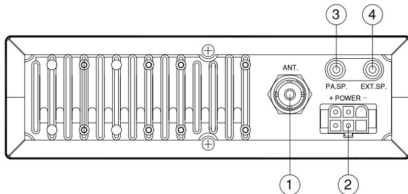
1. **ANTENNA:** This jack accepts a 50 ohms coaxial cable with a PL-259 style plug.
