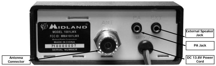
Antenna Connector: Connect a standard 50-ohm CB antenna to this connector.
