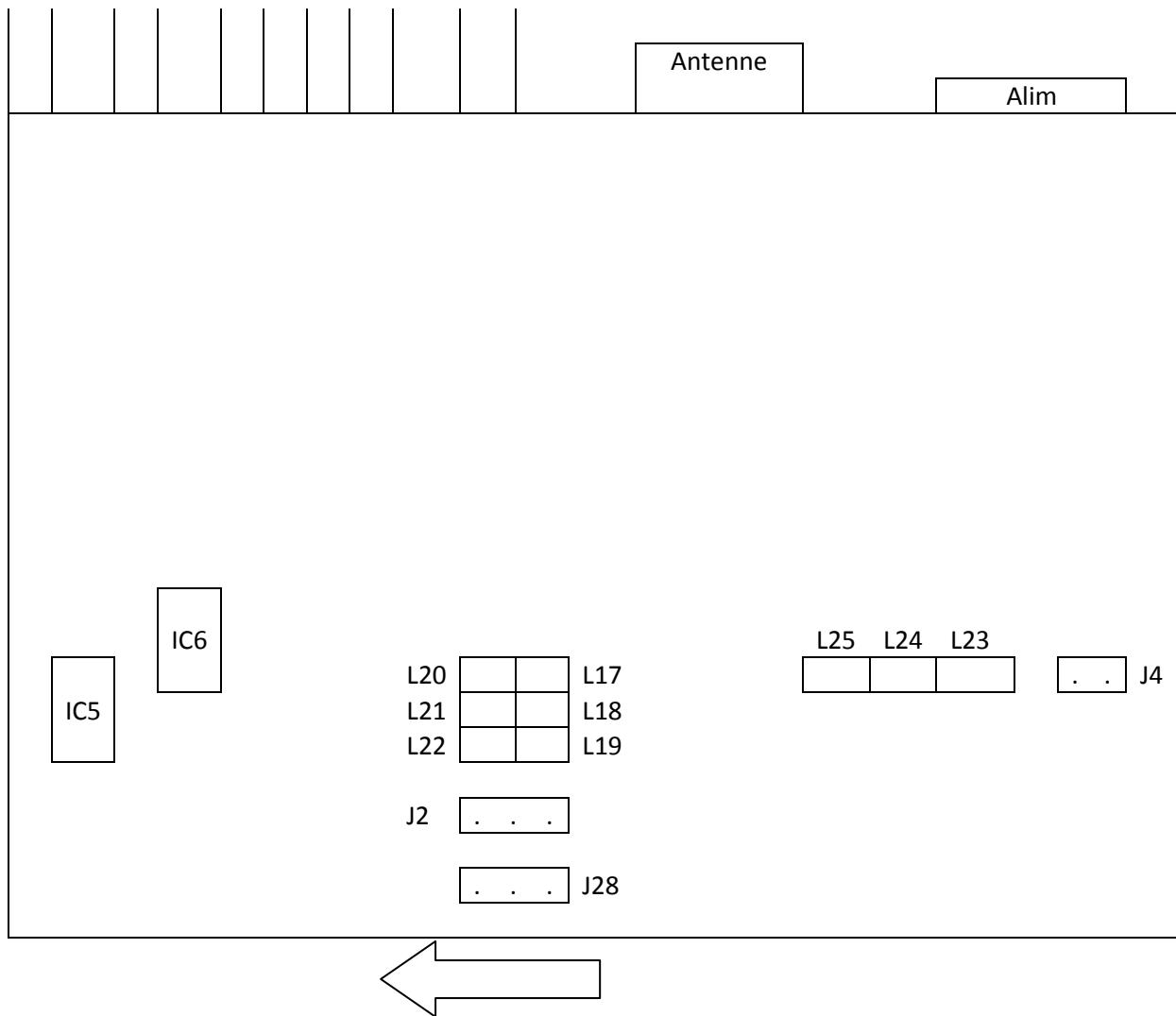
MOVE THE STRAP **J28** OF A NOTCH IN THE SENSE OF THE ARROW
