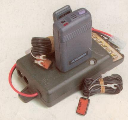
Also used as a pager for radio/cellular phones. Transmits in the 27 MHz band at 0.5 W and AM modulation. Coverage: 200-500 meters.
