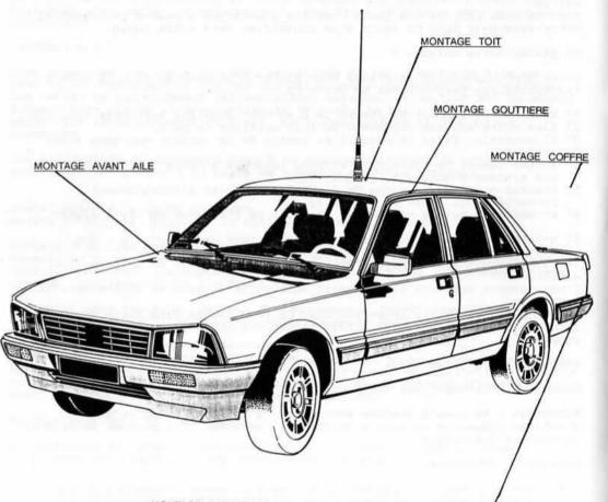
MONTAGE PARE-CHOC (POUR LES VOITURES MUNIES DE PARE-CHOCS METTALLIQUES) PROPAGATION DES ONDES ELECTROMAGNETIQUES FONCTION DE L'EMPLACEMENT DE L'ANTENNE
