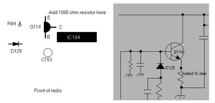
Solder the other end of the resistor to the Emitter leg of Q114.
