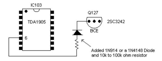
NOTE: Use a 10k ohm resistor if you only use the internal speaker. Use a 100k ohm resistor if you use a external speaker.
