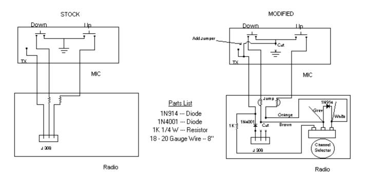
NOTE: If the Up / Down buttons work backwards, exchange the Orange and Brown wires.
