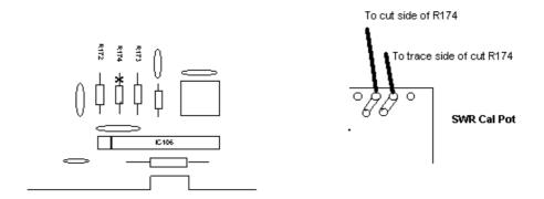
Remove the White and Brown wires from the SWR CAL pot.
