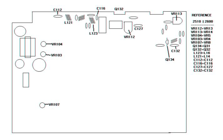
9). Connect power to the radio, and following the alignment procedures, adjust the bias of Q132 to 80mA + -5mA by adjusting VR112.
