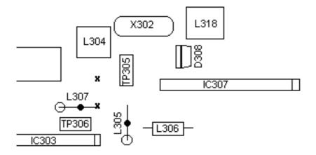
The VCO range is extended by connecting a 180 to 220pf Capacitor between the two pointsmarked "x".
