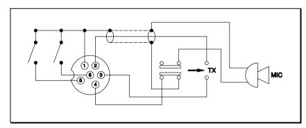
Transceiver Microphone Schematic Diagram
