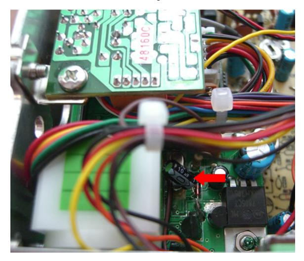
Some SR-490HP radios sold in late spring 2008 had a capacitor installed behind the channel selector. With the capacitor installed the dimmer will only dim a total of two stages instead of three. Clipping one leg of this capacitor will restore the radio to normal three stage dimmer operation. You can see in the above picture that one leg of the capacitor has already been clipped. The red arrow in the above picture points to the blue 10 uF capacitor in question.
