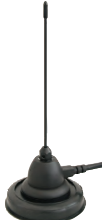
TAXI Mag PR6002: BNC plug PR6116: PL plug for LCmobile UHF-COM and MiCo UHF-COM 440-480 MHz UHF mobile radio antenna, max. 50 Watts, with magnetic base Ø 60 mm, whip: 12 cm, 5 m cable
