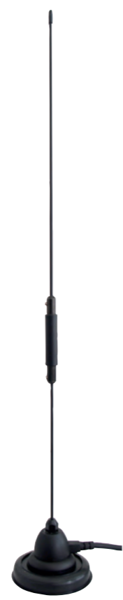
TaxiMag Kit TX4 PR6004: BNC plug PR6115: PL plug for MiCo VHF-COM & LCmobile VHF-COM 136-174 MHz VHF mobile radio antenna, max. 50 Watts, with magnetic mount Ø 60 mm, whip: 51 cm, 5 m cable with plug
