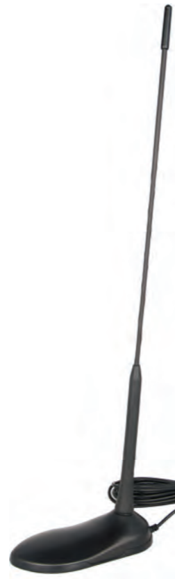
Tornado MAG V/U PR6652 middle freq.: 144-430 MHz, VHF/UHF mobile radio antenna, max. 50 W / 160 W peak, with magnetic base 60x125 mm, whip: 41.5 cm, 5 m cable with PL plug
