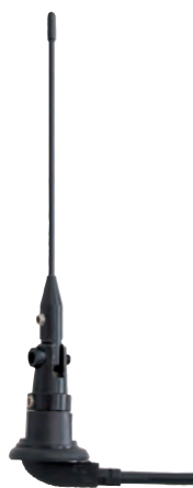
BodyMount PR6001 440-480 MHz UHF mobile radio antenna for fixed mounting, whip: 12 cm, angle adjustable, max. 50 Watt, 5 m cable with BNC plug
