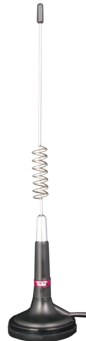
MiniMag-VHF PR6011 136-174 MHz VHF mobile radio antenna with magnetic base Ø 68 mm, whip: 29 cm, 3.8 m cable with PL plug for MiCo VHF-COM & LCmobile VHF-COM
